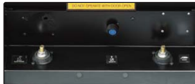
Separate output studs for stick and TIG keep both stick electrode holder and TIG torch connected at the same time — eliminates set-up changeover when switching processes.
